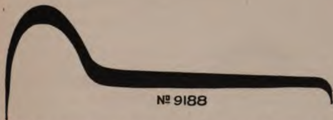
WEAR OF SCHOEN STEEL WHEELS ON BROOKLYN RAPID TRANSIT R.R.
